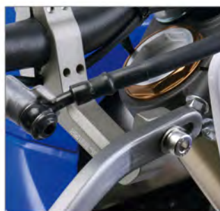
Removed sharp edge to reduce cable damage.
