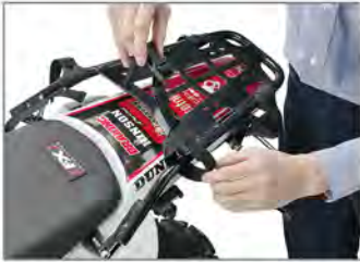
Attach the supplied loading belts to the rear carrier or other frame. (4 places).
