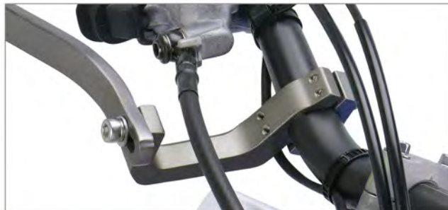
Removed sharp edge to reduce cable damage.
