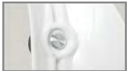
Integrated lower fork guard and lock pin for rigidity and reduced weight.
