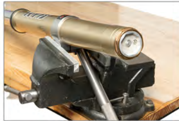
Can be used with a vise when removing the clamp lever.
